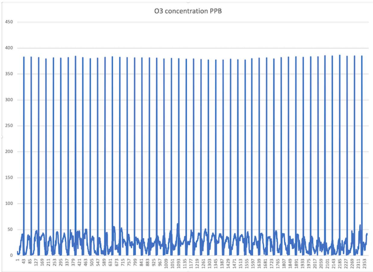
**In the above graph the relative ozone concentrations can be seen as well as the normal diurnal effect. Because 1/2 hour SRECs were used to generate the graph, the daily span check can also be seen at the 10-minute mark (this site was using the common 20 minute zero, 20 minute span settings). This allows a quick check of the instrument operation and span stability.**
