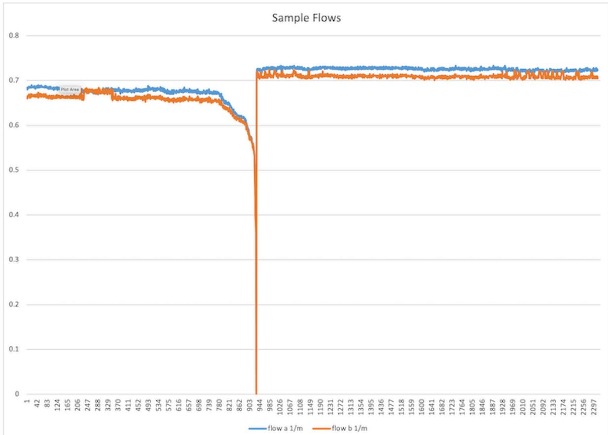
**It can be seen from this graph that the initial flows were around 660/670 cc/min, dropped down to less than 500 cc/min, then suddenly jumped up to 710/720 cc/min when, obviously, the pump or pump diaphragm was replaced. Since the ozone analyzer is not flow dependant, these changes should not affect the readings. Normal flow readings are between 650 and 750 cc/min.**
