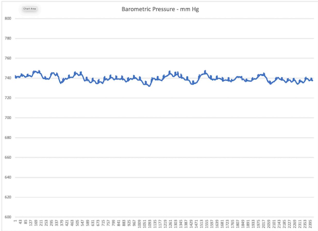
**The pressure reading is generally 20 to 60 mm Hg below the local barometric pressure. The pressure reading will decline slightly over time due to loading on the inline sample filter. This is sometimes a good indication that the filter needs to be changed. Fluctuations in the readings are generally due to normal variations of the barometric pressure.**
