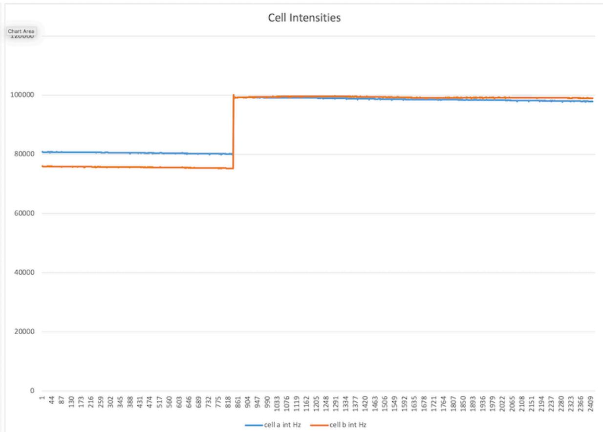
**Within limits, the cell intensities do not affect the instrument readings. However, we recommend keeping them within the range of 70,000 to 110,000. Using the example above, because of normal aging of the photometer lamp, the intensities had slowly dropped to 75,000/80,000, so the lamp power was adjusted (see next graph) to bring the intensities close to 100,000, and then a Detector Calibration was performed to make both intensities equal to 100,000.**
