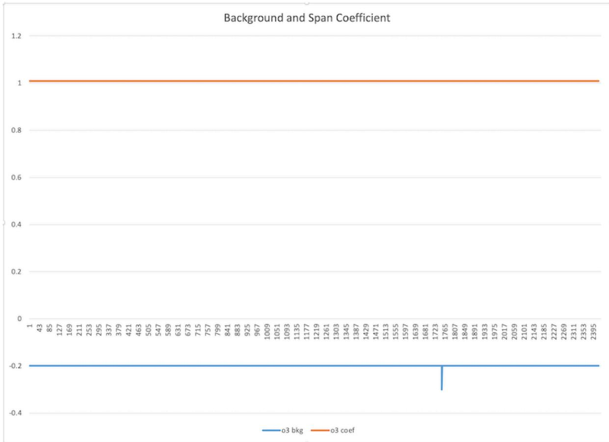
For qa/qc purposes, graphing the background and span coefficient is very useful. The span coefficient should always be close to 1.00 and should rarely, if ever, change. From the factory, the coefficient is usually between 0.98 and 1.02. The background is also quite stable and usually close to zero. From the factory the background is usually between 2 ppb and -2 ppb, but can vary from 5 ppb to -5 ppb.
