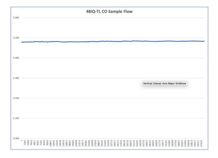
The flow of the 48iQ is controlled by a capillary to be approximately 1.0 LPM for the standard 48iQ and 0.5 LPM for the 48iQTL. Small variations to the flow will not affect the reading, but it is advised to occasionally graph the flow to verify that the pump is operating properly and there are no large leaks. Please note that the flow path of the 48iQTL contains additional components such as a Sample/Zero Valve, a Zero Scrubber and a Permeation Dryer.
