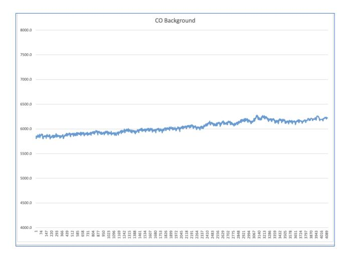
As the correlation wheel deteriorates and the S/R Ratio drops, the CO background concentration slowly increases and should be manually adjusted at least weekly. This data is from a trace level 48iQ and shows the increase to the Background reading as it is automatically adjusted every 4 to 6 hours. The internal zero scrubber option can also be ordered for the standard 48iQ. The graph shows that the CO background increased about 400 ppb over a 12-week period. This would be about 35 ppb per week.
