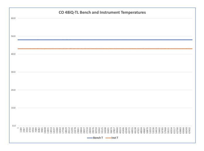
Temperature stability is very important for the 48iQ. The optical bench is tightly controlled to 48°C and with the 48iQTL, the internal case is also controlled to 43°C. It helps if the room, or trailer, that the CO analyzer is operating in is temperature controlled, such as 21°C +/- 2°C. Care should be made that the heater fan or air conditioner output does not blow directly onto the analyzer case.
