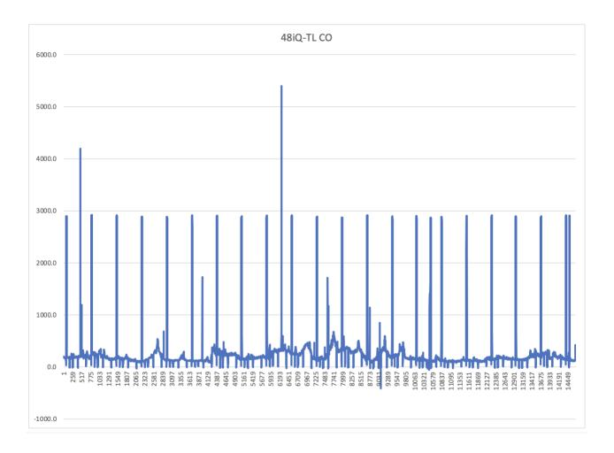
The data for the above graph is from a 48iQ-TL. The graph shows the daily zero/span cycles as well as the auto-zero cycles of the trace level analyzer, which are usually set to occur every 4 or 6 hours. Some of the brief random spikes are probably from nearby sources such as cars or trucks. The normal ambient readings are in the range of 150 to 350 ppb.
